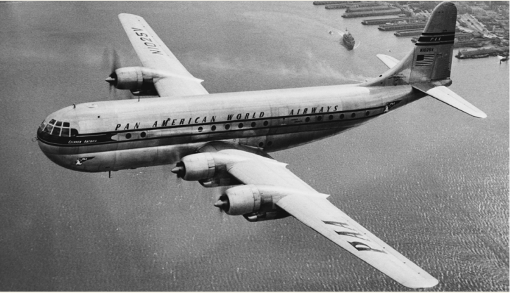
Figure 7. During the latter part of World War II, Boeing developed the C-97 freighter based on the B-29. Post-war, the C-97 was turned into the B-377 Stratocruiser. The similarities with the B-29 are obvious. The Stratocruiser was not successful as an airliner. Credit: Getty.
