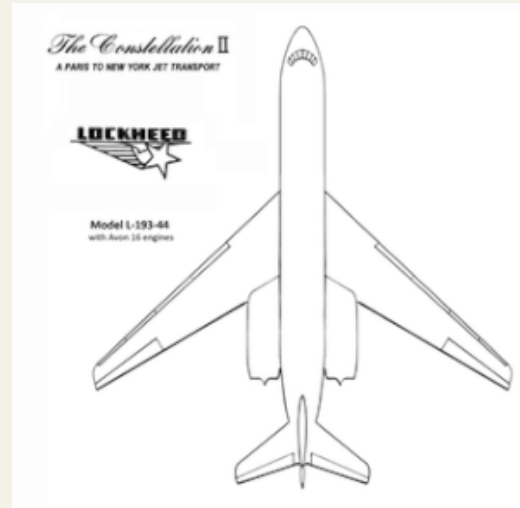
Figure 8. Lockheed proposed a jet tanker for the U.S. Air Force with the internal name L-193. Jets were buried next to the plane's fuselage. A commercial version called the Constellation II was floated. Neither went into production. Credit: Lockheed.
