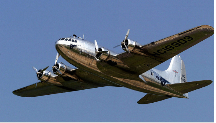
Figure 5. Boeing followed the B-17 with the civilian B-307 Stratoliner, using the engines, wings and tail. Credit: Getty.
